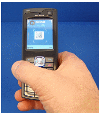
Fig.3 Capture of 2D Barcode in Reader Application
