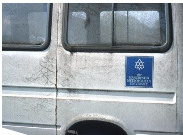
Fig 1: Biofilms and deterioration
